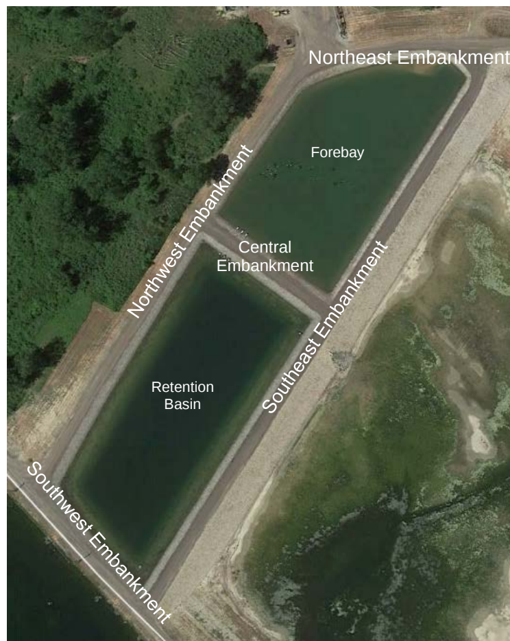
Figure 5. Forebay and Retention Basin Embankment Terminology
