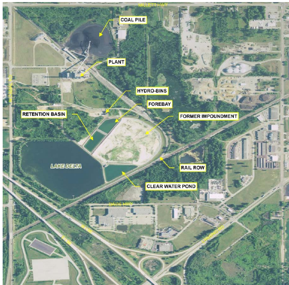
Figure 2. Erickson Power Station Site Configuration
