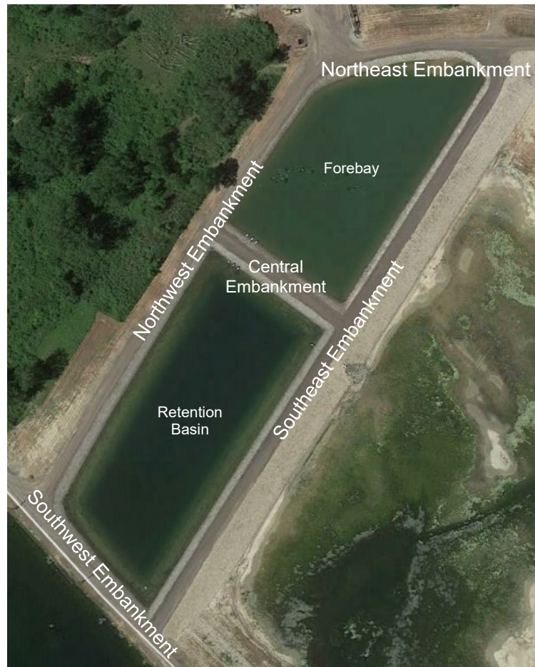
Figure 4. Forebay and Retention Basin Embankment Terminology
