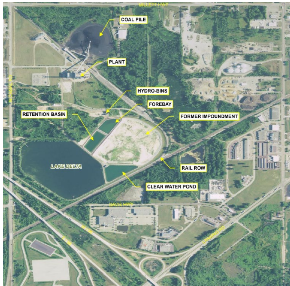
Figure 2. Erickson Power Station Site Configuration
