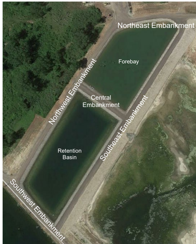
Figure 4. Forebay and Retention Basin Embankment Terminology
